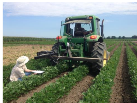
Figure 2 Field on-the-go system hyperspectral imaging system.
